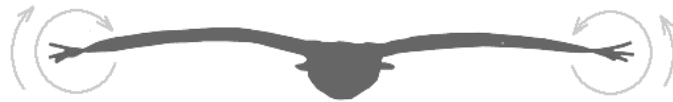
Figure 13. View on a flying goose and the upwash left and right of it.
