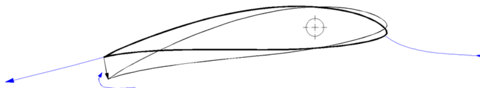
Figure 18. Possible tendency to flow around the trailing edge of the profile with rapid increase in the angle of attack around a far forward positioned axis of rotation.
